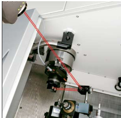
Fig. 4. Renishaw RX-10 setup for vertical axis roll errors
