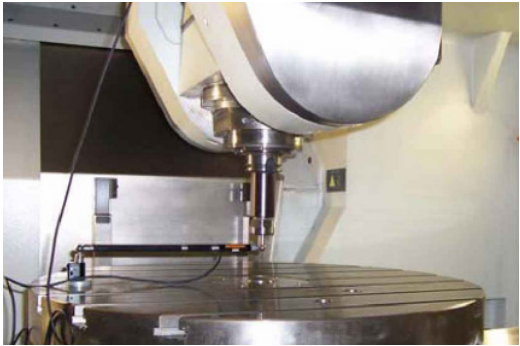
Fig. 5. DBB setup for rotary joint errors
