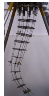
Fig. 2. The flexible structure of the robotic unit
