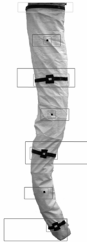
Fig 7. Markers detection. With darker color is indicated the search region. With lighter color are labeled the found markers.
