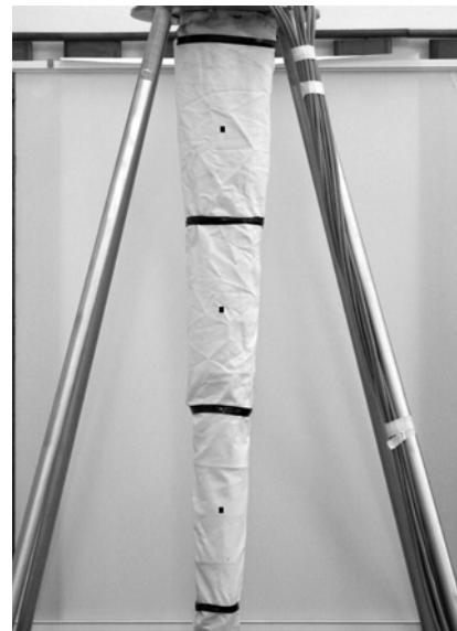
Fig 5. Black lines mark the extremities of segments. Critical points are extracted as the center of mass for each black line
