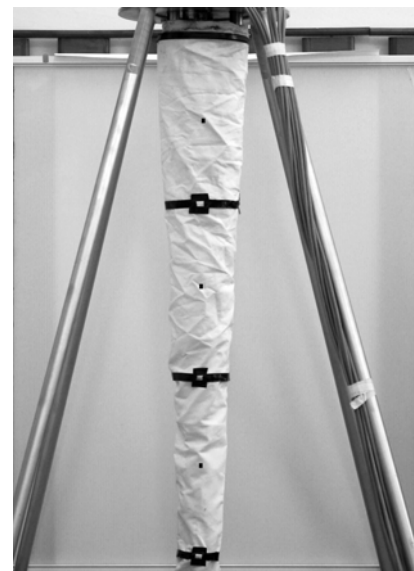
Fig 6. New set of markers which able de artificial vision system to identify the critical points, but also if the twist phenomenon occurs.
